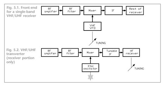
bandwidth of the IF circuits, a modern transverter is very similar to a transceiver front-end for the same band. The advantage of transverting is that it provides all the facilities of the HF rig on the VHF or UHF band, and allows extra bands to be added at modest cost compared with a range of new single-band rigs. The disadvantage is that receiver performance may be compromised, especially with strong signals.
