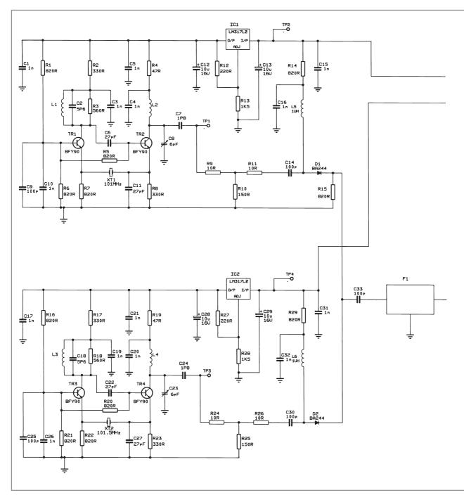
Fig. 10.5. Circuit of the 404/406MHz local oscillator for the 432MHz transverter
