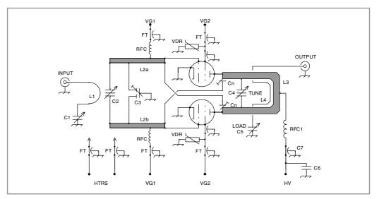
Fig. 8.22. Circuit of the W1SL power amplifier. See Fig. 11.5 for additional screen-grid protection components
