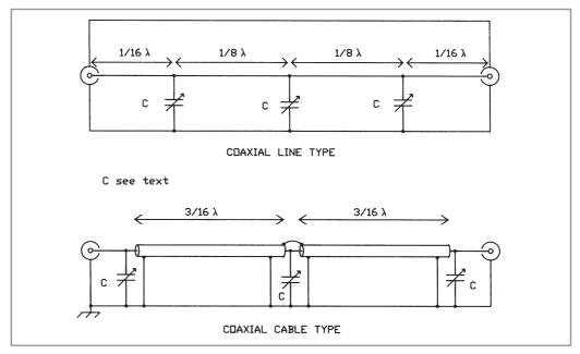
Fig. 12.20. Impedance matching units for VHF/UHF
