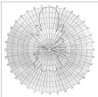
Fig. 7.2a. Polar pattern of a long-Yagi antenna, linear dB scale. Minor lobes are excessive, because the antenna is being operated below its design frequency
