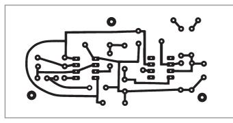
Fig. 9.23. PCB mask for the 50MHz ALC amplifier board (underside view; single-sided board)
