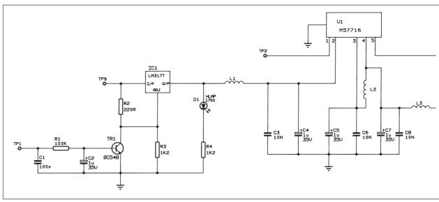
Fig. 10.11. Circuit of the 432MHz modular PA and VSWR/power meter
