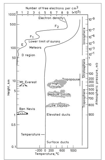
Fig. 2.10. The lower and upper atmosphere, showing the troposphere and the regions of the ionosphere. The logarithmic scale of height compresses the upper portion of the diagram. At the same scale as the lowest part, the whole diagram would be tens of metres high!
