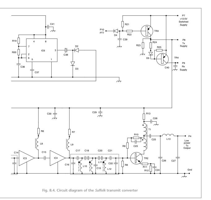
wanted mixer output at 144MHz will be -19dBm. To reach a final output of 10W (+40dBm) thus requires a gain of very nearly 60dB, and such high gain in the same frequency range can be the cause of instability. The use of MMIC amplifiers, negative-feedback amplifiers and intentional loss between stages allows the required gain to be achieved with stability.
