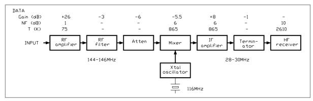
Fig. 5.3. Block diagram of the *Suffolk* transverter for 144-146MHz (receiver portion only) with input data
