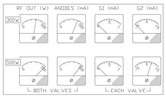
Fig. 6.11. Meter readings for a two-4CX250B amplifier, correctly set-up for 300W and 500W RF output power. The RF output and anode current readings are for both valves combined, while the G1 and G2 currents are for each valve
