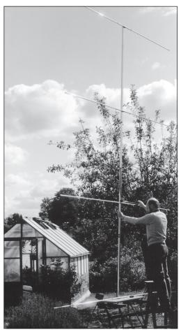
Fig. 9.43. Adjusting the VSWR of the 4-element Yagi for 50MHz, with the antenna pointing straight up. No further adjustment was needed after the antenna was installed.
