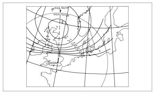
Fig. 2.25. Isoflectional map for a station in London. The contour marked  $0^{\circ}$  joins locations where the auroral reflection would be most favourable, if ionization is present at E-layer heights. The same map would apply to field-aligned ionization
