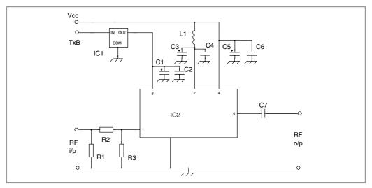
Fig. 9.7 shows the circuit diagram for the PA, including the bias control circuit. Switching between transmit and receive is by applying the bias; the supply to the collectors of the transistors is permanently connected. The TXB (switched 12–13.5V transmit) line used to power the transmit converter also switches the supply to the 78S09 bias regulator IC1.
