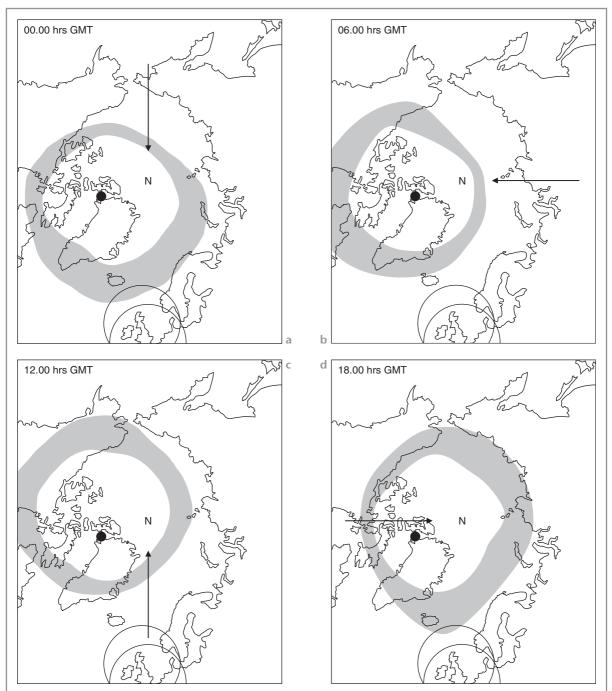
Fig. 2.22. The position of an auroral oval at six-hourly intervals during the day. The geomagnetic north pole (shown by a dot) rotates about the geographic north pole in the centre of each picture, and the direction of the solar wind is shown by an arrow. The result is that the auroral oval approaches and recedes twice a day. Rings show the accessible range from London and Edinburgh
