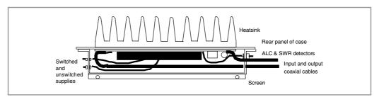
Fig. 8.17. Mounting the M57713 amplifier to the rear panel of the transverter case. Note the 'U' shaped metal screen, and that the PA module is mounted directly on the heatsink through a cut-out in the rear panel
