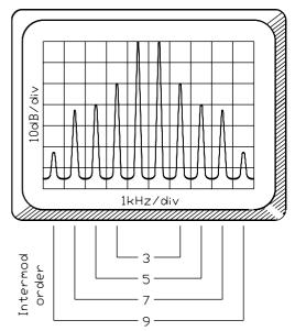
Fig. 6.2. Intermodulation products from a real-life SSB transmitter grossly overdriven by the same tones as in Fig. 6.1. IPs beyond 9th-order will undoubtedly be present too, further increasing the signal bandwidth
