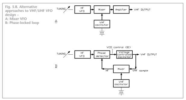
resulting output to a suitable level. Examples of transceivers using this technique are the old TS700 and the IC201. Mixer VFOs offer many opportunities for oscillator noise. The mixer cannot be run at too high a level without producing spurious products, and at the output of the mixer the carrier level can sink perilously close to the circuit noise. Any subsequent amplification of the low-level carrier also brings up the accompanying noise.
