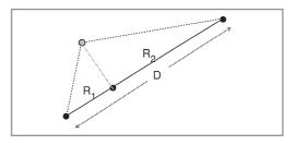
Fig. 2.14. A path with an intermediate reflection
