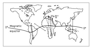
Fig. 2.41. The longest-distance TEP paths on 144MHz have been symmetrical about the geomagnetic equator
