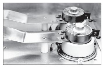
Fig. 6.8. Above-chassis neutralizing flags for a W1SL amplifier (Chapter 8)
