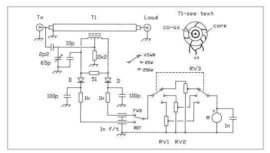
Fig. 12.11. VSWR/power meter suitable for 28–144MHz
