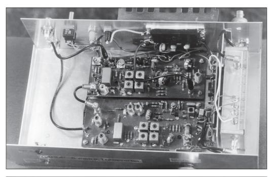
Fig. 9.12. Rear view of a prototype G4HUP 50MHz transverter. The recommended heatsink is larger than the one shown here.
