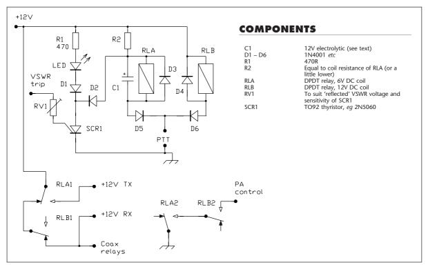
Fig. 11.14. A simple transmit/receive sequencing circuit for use with Fig. 11.12
