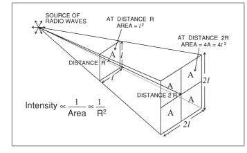
*radio propagation path* is the route taken by the wavefront as it travels from the transmitting to the receiving antenna. The attenuation along the path is known as the *path loss*.
