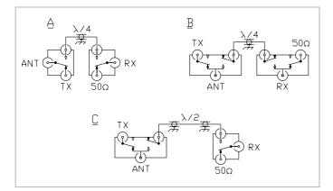
Fig. 11.13. The optimum length of cable between the two coaxial relays depends on their construction
