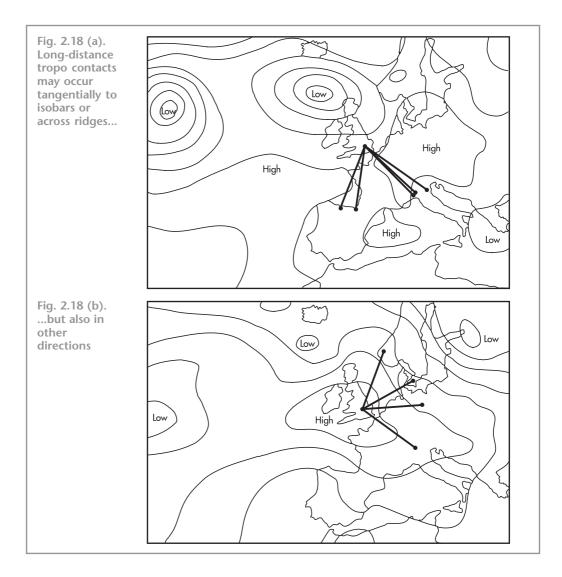
much shallower. This is borne out by the observation that while tropo ducting may occur many times a year on the 144MHz band, there are very few records of tropo ducting at 70MHz or lower frequencies in the UK. It also explains why strong ducted signals can be found on the 432MHz or microwave bands at times when ducting on 144MHz is much weaker or even absent.
