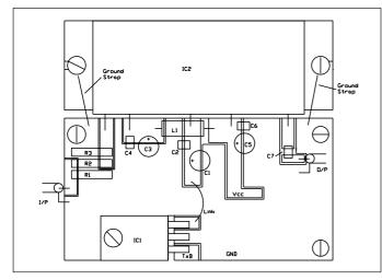
Fig. 9.19. Component layout for the 50MHz PA board
