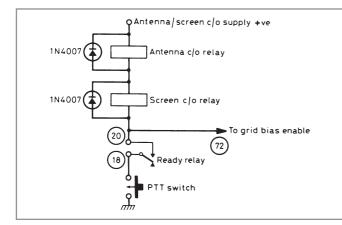
Fig. 11.10. 'Ready' relay logic for the comprehensive PSCU [4]. Fig. 11.15 shows another option
