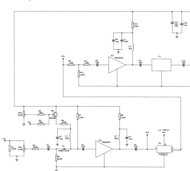
Fig. 10.8. 28–432MHz transmit-converter circuit
