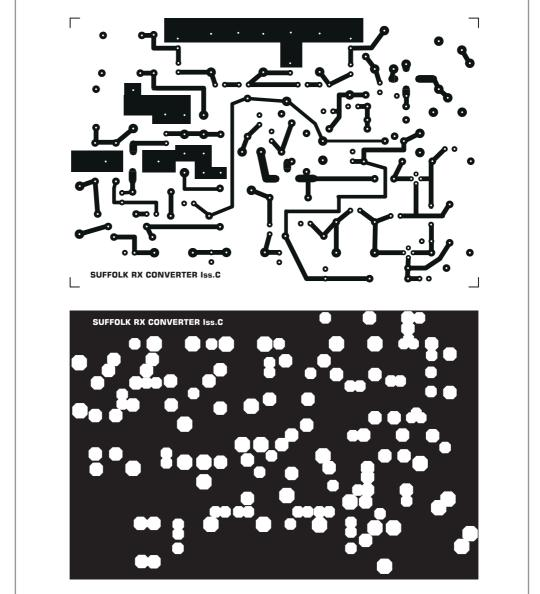
Fig. 8.9(a). Full-size PCB mask for the receive converter (underside)
