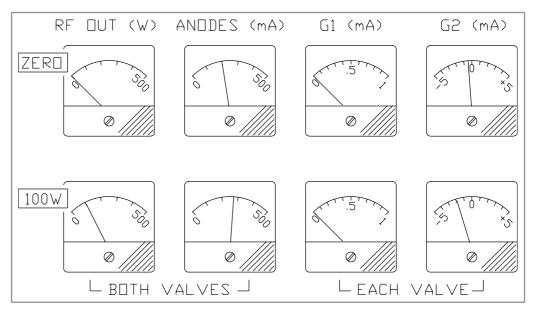
Fig. 6.10. Meter readings for a two-4CX250B amplifier, correctly set-up for standing current (zero RF output power) and at 100W RF output power. The RF output and anode current readings are for both valves combined, while the G1 and G2 currents are for each valve
