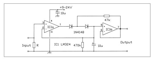
Fig. 12.22. Circuit to convert a wattmeter or VSWR meter to indicate PEP
