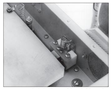
Fig. 10.19. Close-up of the end of the anode line. The output flapper capacitor and its safety RF choke are mounted on a PTFE block. Also visible are the HV RF choke (top left), the screened blower inlet and the tuning flapper (bottom centre)
