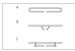
Fig. 7.16. Three methods of matching a driven-element to  $200\Omega$  balanced, for use with a half-wave balun (Fig. 7.15). If the driven element impedance would be  $50\Omega$ , a simple folded dipole (A) can be used. The Delta-match (B) and T-match (C) are adjustable
