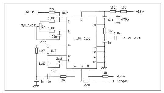
Fig. 12.27. LA8AK's audio up-converter for CW meteor-scatter
