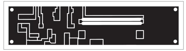
Fig. 10.12. Full-size PCB layout on the top-side of the 432MHz PA/VSWR board. The underside of the board is a continuous copper groundplane
