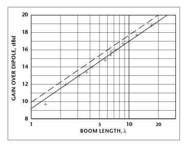
Fig. 7.5. Yagi antenna gain versus boom length.
