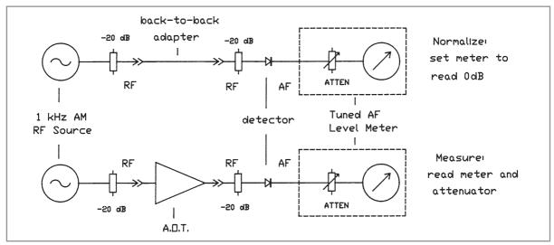
Fig. 12.16. Using a tuned audio-level meter to measure the gain of an amplifier
