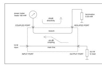
Fig. 12.9. Power measurement using a directional coupler
