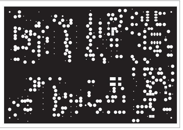
Fig. 9.30b. Top side of the transverter PCB
