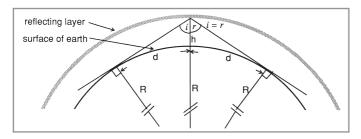
Fig. 2.11. The geometry for maximum range using a change of direction at a height h. Note the possible range extension if the antenna is significantly above ground level (not to scale)
