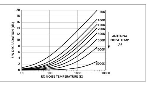
Such a small improvement may scarcely be noticeable on the air, except at the very limits of weak-signal working such as moonbounce. In other words, if the receiver noise temperature is as low as the minimum probable noise temperature of the antenna, the receiver is about as sensitive as it needs to be for terrestrial work. On the lower VHF bands, manmade noise can exceed galactic and ground noise by 10dB or more, so there's absolutely no need for very low noise figures on 50 or 70MHz.
