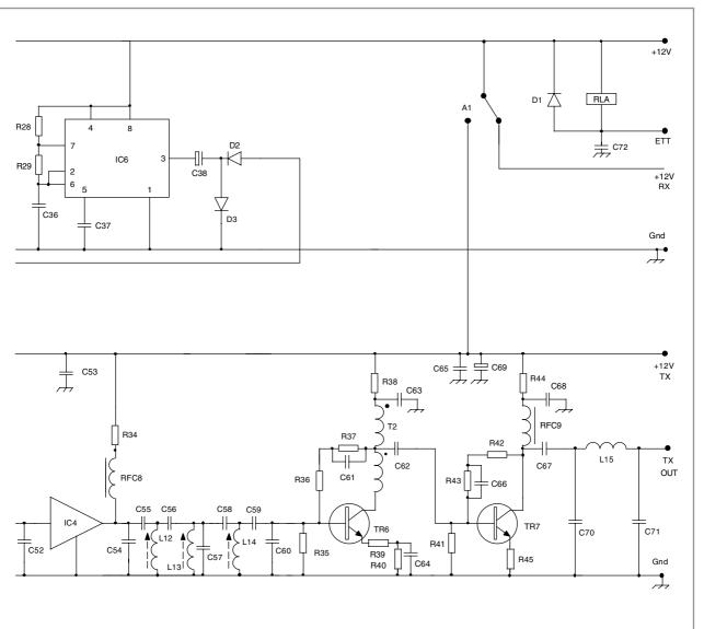
Fig. 9.27. Circuit of the 70MHz transmit converter and ALC generator
