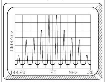
the signal frequency to the intermediate frequency. The signal is at  $f_1$ ,  $f_2$  is the LO and  $(f_1-f_2)$  is the IF; in this particular case the filter is intended to select only the IF. The mixer stage has to be a non-linear device, or else it wouldn't work; but its non-linearity can often let in a host of further intermodulation problems.
