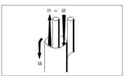
Fig. 7.13. Currents flowing on the inside and outside of a coaxial cable. Currents I1 and I2 on the inside of the cable are always equal. If the system is unbalanced, a current I3 will flow on the outside of the outer sheath
