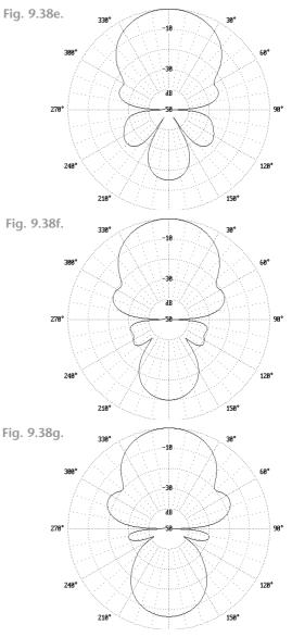
Fig. 9.38a-g. The rearward pattern of a short Yagi changes rapidly with less than  $\pm 1\%$  change in frequency. The Yagi can be tuned to place the optimum patterns for interference rejection (c-d-e) in the DX segment of the band.
