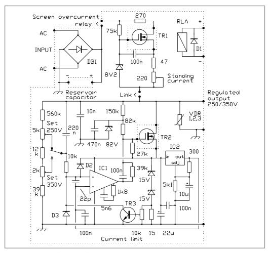
Fig. 11.2. Screen voltage regulator for a single 4CX250/350, by G4JZQ. Relay switching is provided between output voltages suitable for Class C and Class AB1, and each voltage is adjustable. Large dots show interfaces to a PC board
