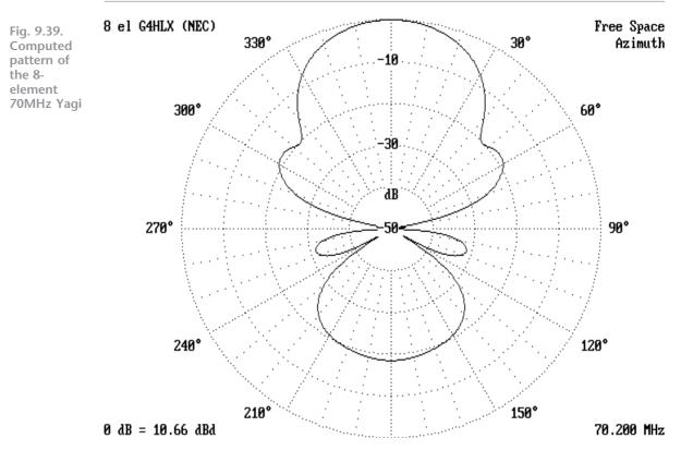
split becomes deep and the front/back ratio is very high. A small further increase in frequency produces a new 'HF' rear lobe (Fig. 9.38d) which rapidly grows outwards at 180° (Figs 9.38e-f-g), while the remains of the old 'LF' backlobe wither away. Meanwhile the forward gain has been gradually increasing with frequency, although it will eventually begin to drop very sharply. If you go even further HF, the first director will begin to act as a reflector, and the antenna beams backwards!
