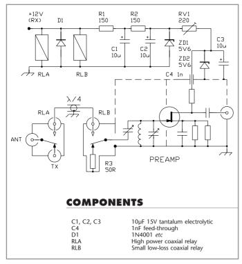
Fig. 11.12. Coaxial-relay switching and DCsupply precautions to protect a GaAsFET preamplifier
