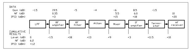
Fig. 9.2. TCALC analysis of the 50MHz receive converter and HF receiver
