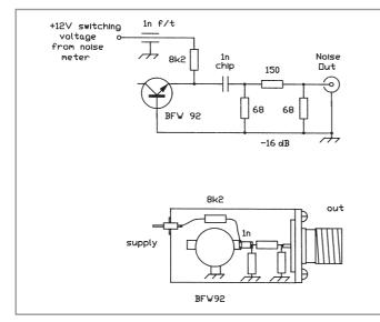
Fig. 12.19. Circuit and arrangement of the noise head using a BFW92 transistor
