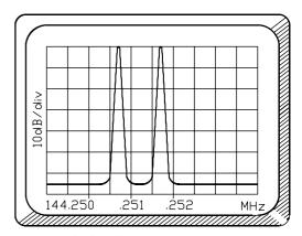
Fig. 6.1. Idealized output from an SSB transmitter with a suppressed carrier frequency of 144-250000MHz, fed with pure sine-wave tones of 700Hz and 1700Hz
