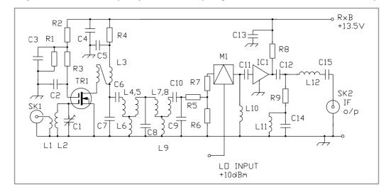
Fig. 9.3. 50MHz receive converter circuit Fig. 9.4. 22MHz local oscillator for the 50MHz transverter (on same board as receive converter)
