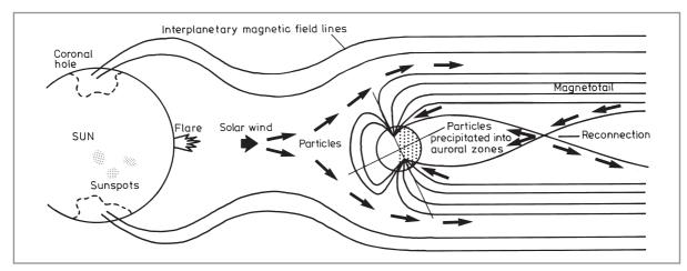
Fig. 2.21. Solar interactions with the earth's magnetic field (not to scale). The earth's magnetic field is pushed away from the day side by the solar wind. Note the magneto-tail containing trapped charged particles, extending away from the earth on the night side
