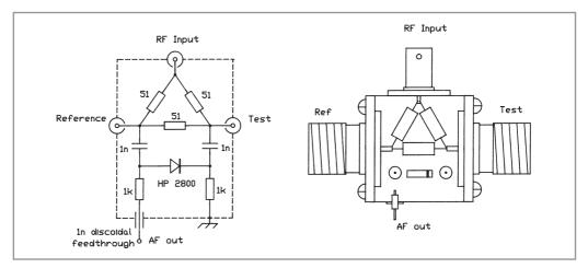
Fig. 12.13. Construction of the return-loss bridge
