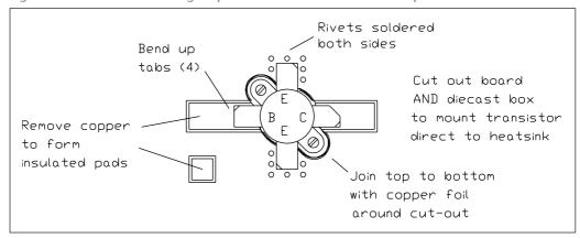
Fig. 9.37. Method of mounting RF power transistors and other components
