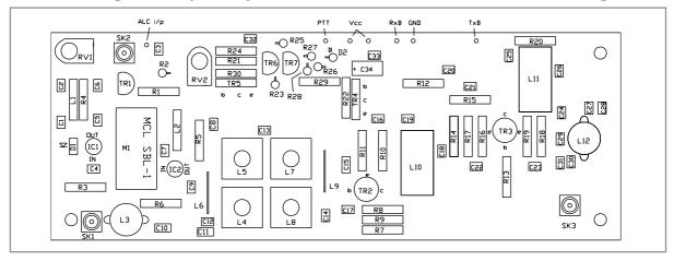
Fig. 9.17. Component layout for the 50MHz transmit converter, driver and switching board
