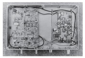
Fig. 9.31. Photograph of a prototype *Cray* transverter assembled in a die-cast box
