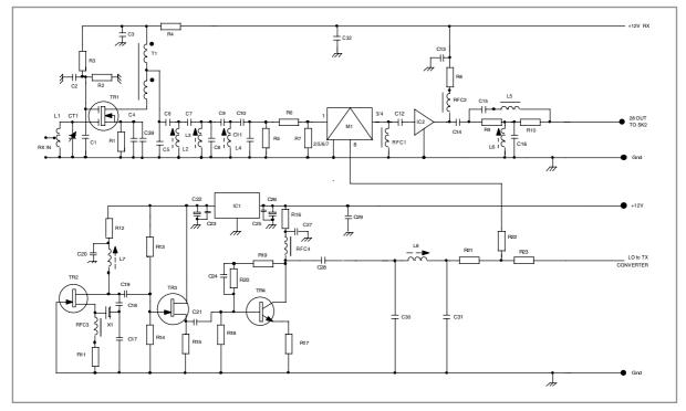
Fig. 9.26. Circuit of the 70MHz receive converter and local oscillator
