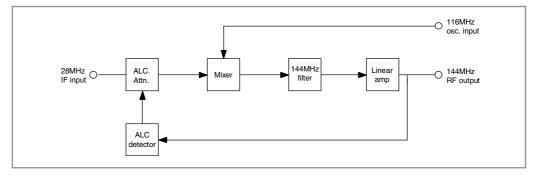
Fig. 8.3. Block diagram of the Suffolk transmit converter
