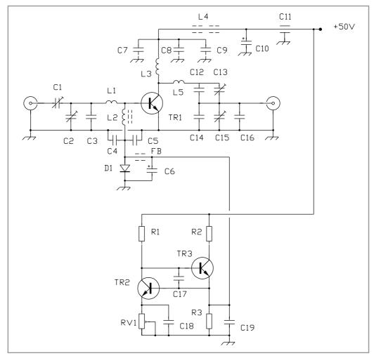
Fig. 9.36. Circuit for 50MHz and 70MHz power amplifiers by G3XBY
