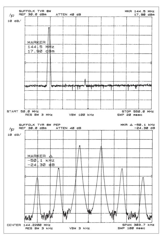
attenuation will retain the same system noise figure, with an improved overall system IP3 of -2dBm. Alternatively an attenuation of 8dB will reduce the system noise figure to 2dB with the same IP3 as the original converter. Notice how sensitive the overall performance is to very small changes in gain. As this and other new MMICs become available, the choice is yours.
