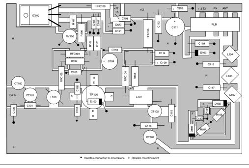
Fig. 9.33. Component layout of the Cray 70MHz power amplifier board
