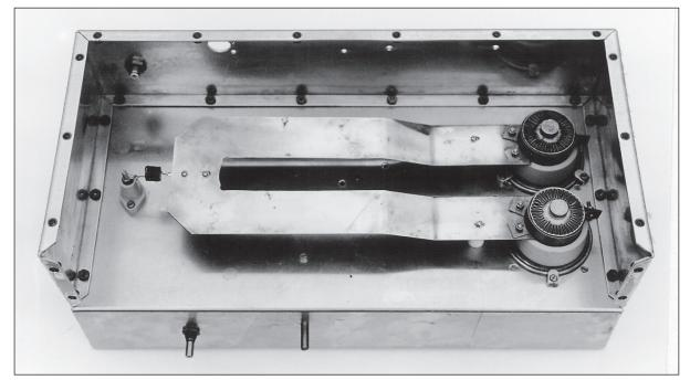
Fig. 8.23. Top view of a partly-constructed W1SL amplifier. Still to be added are the front panel, anode-tuning capacitor, output coupling and top cover
