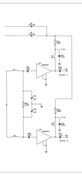
switching if desired. A helical filter at 404MHz selects the desired fourth harmonic and attenuates all other signals to -50dBc typical. As with the other parts of the transverter, using a pre-tuned filter makes complicated testgear unnecessary. The output of the filter feeds a Wilkinson power divider, each output of which is followed by an MSA0304 MMIC. These provide the gain required to produce two output signals of +10dBm at 404MHz.
