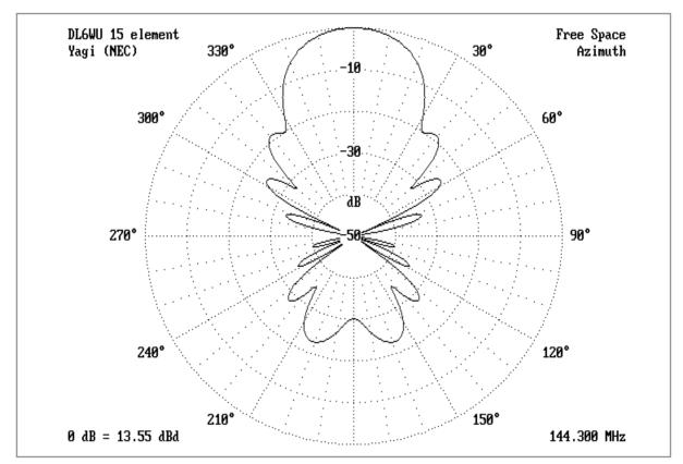
Fig. 8.31. E-plane pattern of the 15-element DL6WU Yagi, calculated by the NEC program. The front/back ratio should be about 30dB, and the first sidelobes should be about –18dB relative to the main lobe
