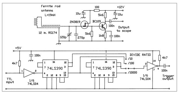
Fig. 12.6. MSF phase-comparison unit
