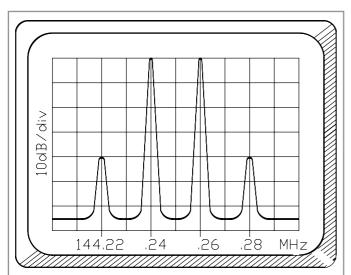
Fig. 5.5. Spectrum analyser display of thirdorder intermodulation between signals on 144-240MHz and 144-260MHz. The intermodulation products appear on 144-220MHz and 144-280MHz
