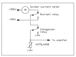
Fig. 11.4. Screen-grid metering, changeover switching and run/set switching within the PSCU (one for each grid). Fig. 11.15 shows an alternative system with SCR 'crowbar' protection for the screen grids
