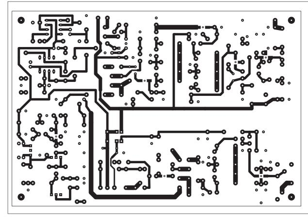
Fig. 9.30a. Full-size PCB track layout of the Cray 70MHz transverter board, underside view
