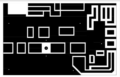
Fig. 9.32. Full-size PCB track layout of the *Cray* 70MHz power amplifier board (top view; underside is un-etched copper groundplane)
