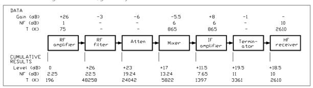
Fig. 5.4. Full noise/gain analysis of the Suffolk transverter
