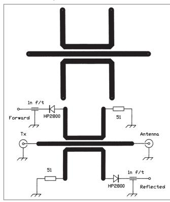
formed from parallel transmission lines, and those such as the Bruene bridge based on current transformers. Both give outputs proportional (in some fashion) to the forward and reflected power in the main line. Simple parallel-line couplers have a frequencydependent sensitivity, so using them on more than one band may not be practical. However, they will work at UHF and above, whereas the practical limit for current-transformer types is the 144MHz band.
