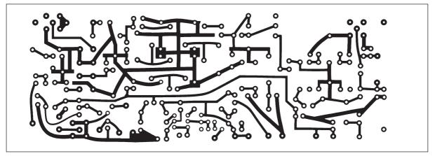
Fig. 9.16. PCB mask for the 50MHz transmit converter, driver and switching board (underside view; top side is un-etched copper groundplane)
