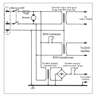
Fig. 11.11. Interconnection to the HV and screen-supply transformers
