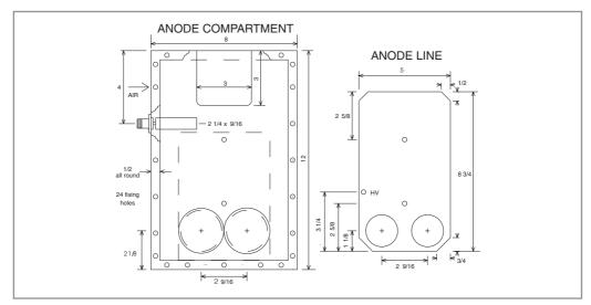
Fig. 10.17. Dimensions of ARCOS K2RIW anode line and anode compartment (dimensions in inches). The size of the large anode-line holes depends on the type of finger stock used
