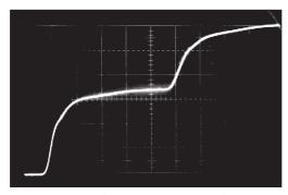
Fig. 12.15. Oscilloscope trace from the Simplest TDR connected to 20m of cable with the far end open-circuited
