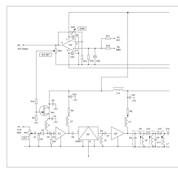
can do little to remove this product, so you are relying on the mixer to avoid generating it at excessive levels. Diode-ring mixers provide the highest level of fifth-order rejection of any type of mixer I tested, but in order to achieve this the IF drive level *must* be kept low.
