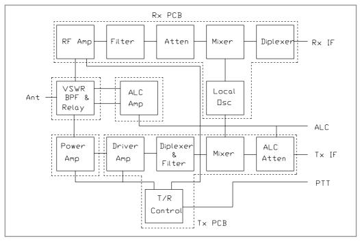
Fig. 9.1. Block diagram of the G4HUP 50MHz transverter, showing division into PC boards
