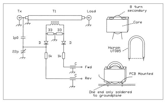
Fig. 12.12. PCB-mounting VSWR bridge using a two-hole ferrite core
