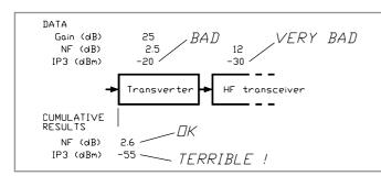
Fig. 5.16. 1970's style transverter and HF transceiver
