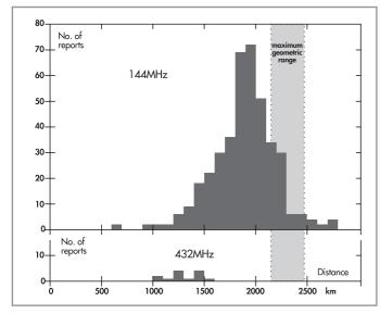
Fig. 2.45. DX operators' maximum ranges by meteor-scatter, taken from the 'Top List' in *DUBUS* 1989/1
