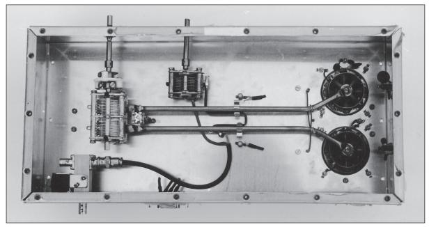
Fig. 8.24. Underside view of a partly-constructed W1SL amplifier, minus its DC wiring
