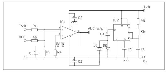
Fig. 9.9. ALC amplifier circuit for the 50MHz transverter
