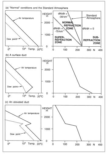
The most common VHF/UHF propagation occurs due to changes of refractive index within the troposphere (Fig. 2.10). There are three types of tropospheric propagation which take signals a significant distance beyond the horizon:
