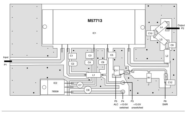
Fig. 8.16. Component layout for the M57713 linear amplifier
