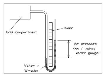
Fig. 6.6. A simple U-tube water gauge for measuring air pressure
