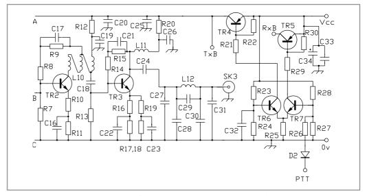
Fig. 9.6. 50MHz driver amplifier and TX/RX switching (on same board as transmit converter)
