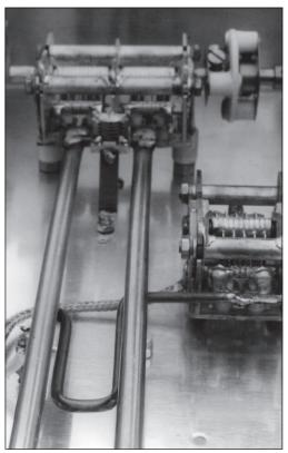
Fig. 8.27. Close-up of the W1SL grid lines and input coupling loop. The two-gang capacitor C2 is mounted on stand-off insulators, and is grounded only by the vertical copper strip from the centre of its frame. The small differential balancing capacitor C3 is connected across the grid lines in front of C2, and also to the grounding strip
