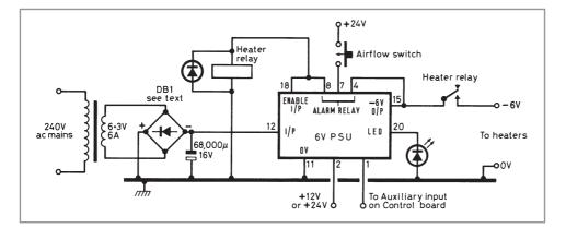
Fig. 11.8. Connections to the heater regulator PC board [6]
