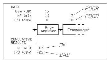
Fig. 5.15. Effect of a preamplifier on a typical 144MHz transceiver. Sensitivity is improved, but the intermodulation intercept becomes much worse
