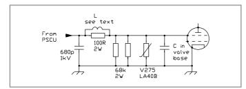
Fig. 11.5. Screen-grid protection circuitry within the amplifier
