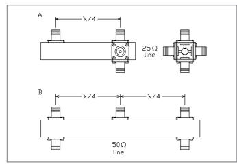
Fig. 7.11. Two types of four-way 50 $\Omega$  power divider: quarter-wave (A) and half-wave (B)
