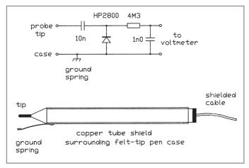
Fig. 12.3. A high-impedance RF probe, suitable for a  $10M\Omega$  voltmeter
