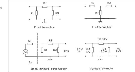
Fig. 12.7. Pi and T attenuators
