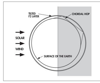
MUF. In fact, the daytime increase in MUF results partly from the pressure of the solar wind on the ionosphere, which results in a lowering and compression of the F region. This produces a higher ionization density and also a more favourable geometry for reflection (Figs 2.21 and 2.40).
