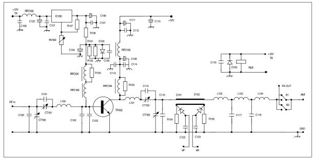
Fig. 9.28. Circuit of the 10W PEP 70MHz power amplifier. All component numbers start at 100
