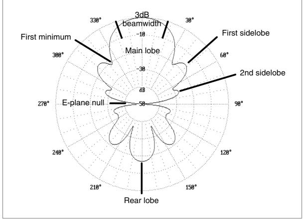
Fig. 7.1. Polar pattern of a long Yagi antenna showing the main features (E-plane)
