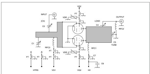
Fig. 10.16. Circuit of the K2RIW 432MHz power amplifier. See Fig. 11.5 for additional screengrid protection components
