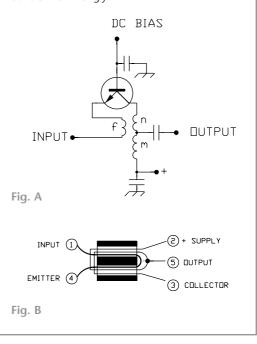
mixer and feedback amplifiers. The target noise temperature of 150K is achieved almost exactly, and with a good HF receiver the dynamic range is very respectable.
