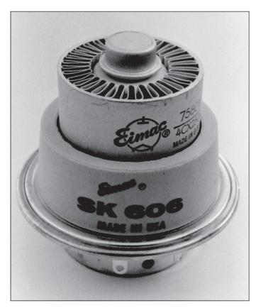
Fig. 6.3. 4CX250R valve in Eimac SK600 base, suitable for frequencies up to 144MHz, with SK606 chimney
