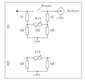
Any system you buy or build will probably start out with too much gain. Commercial preamps need enough gain to produce some improvement on the deafest transceiver. The same applies to transverters: even the ones in this book are designed with enough gain to suit a transceiver with a fairly high noisefigure at 28MHz. Your transceiver may be more sensitive, so you can get rid of the excess gain in the preamplifier or transverter.
