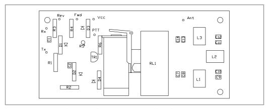
Fig. 9.21. Component layout for the 50MHz VSWR-LPF board
