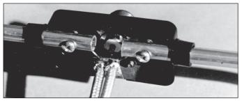
Fig. 7.17. Constructional details of a folded dipole and halfwave balun for 432MHz, using a commercial plastic moulding and an N connector. Fill with closed-cell aerosol foam for waterpoofing
