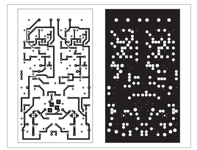
Fig. 10.6. Full-size PCB layout of the underside of the 404/406MHz local-oscillator board. The top of the board is a continuous copper groundplane, etched or counterbored as shown
