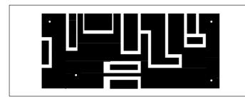
Fig. 9.18. Full-size PCB mask for the 50MHz PA board (top view; single-sided board)
