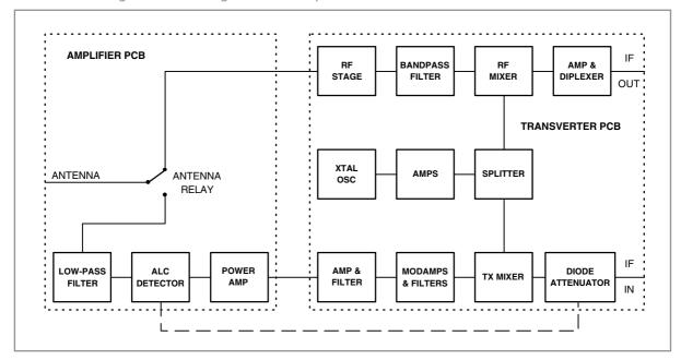
Fig. 9.25. Block diagram of the Cray 70MHz transverter
