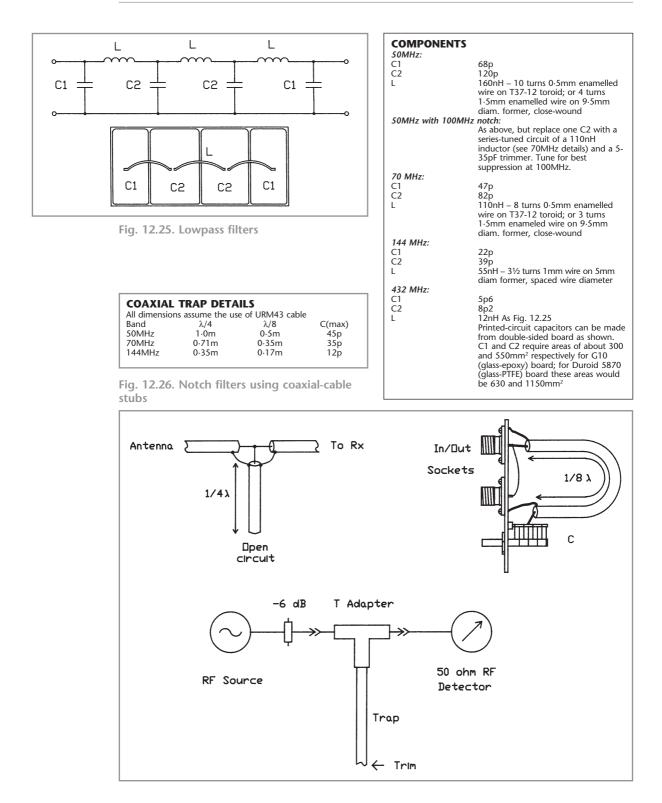
the large circulating currents – and if they don't survive, they weren't "good quality"! For the 432MHz LPF, Fig. 12.25 gives an alternative layout using PCB capacitors.
