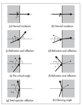
Fig. 2.5. Refraction and reflection at an interface. Left-hand column: wave speeds up. Right-hand column: wave slows down
