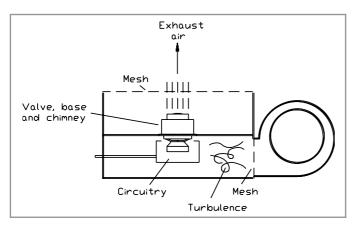
Fig. 6.5. As well as the valve in its airflow socket and chimney, sources of pressure drop in an airflow system include screening mesh, obstructions, turbulence and sharp changes of direction
