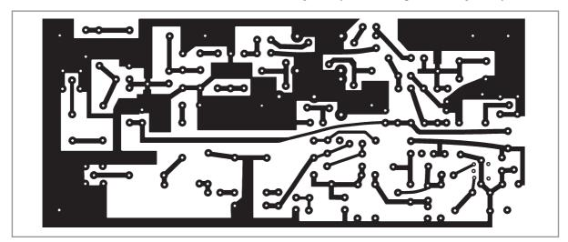
Fig. 9.14. Full-size PCB mask for the 50MHz receive converter and LO board (underside view; top side is un-etched copper groundplane)
