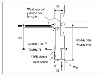
Fig. 9.42. Approximate dimensions (mm) of gamma matches for 50MHz and 70MHz, using the constructional methods described in the text. Adjust for minimum VSWR as shown in Fig. 9.43, and optionally cut off excess rod beyond the clip
