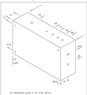
Fig. 9.22. Drilling diagram for the case housing the 50MHz VSWR-LPF board
