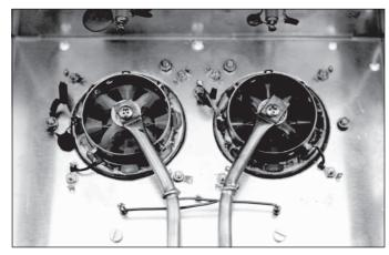
Fig. 6.9. Cross-connection of the neutralizing flags shown in Fig. 6.6 to the opposite grids
