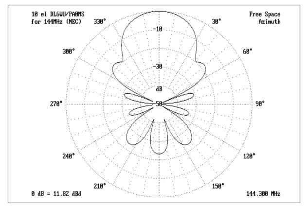
Fig. 8.29. E-plane pattern of the 10-element DL6WU/PA0MS Yagi, calculated by the NEC program. The front/back ratio should be well over 20dB, and the first sidelobes at about – 18dB relative to the main lobe
