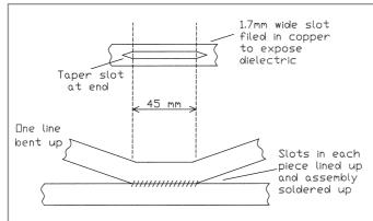
directional couplers, with some practical designs, see [6] and [21]. Directional couplers are usually rather frequency-conscious so you'll need to calibrate them for each band. Generally a coupler which uses parallel lines has an upper frequency limit where the length of the branch line approaches a quarterwavelength. The lowest useful frequency is set by the falling coupling factor.
