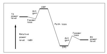
Fig. 4.6. Changes in relative power levels, from transmitter to distant receiver. (Receiving antenna gain does not change the actual power level, but represents collection of power from a wider capture area – see Chapter 7.)
